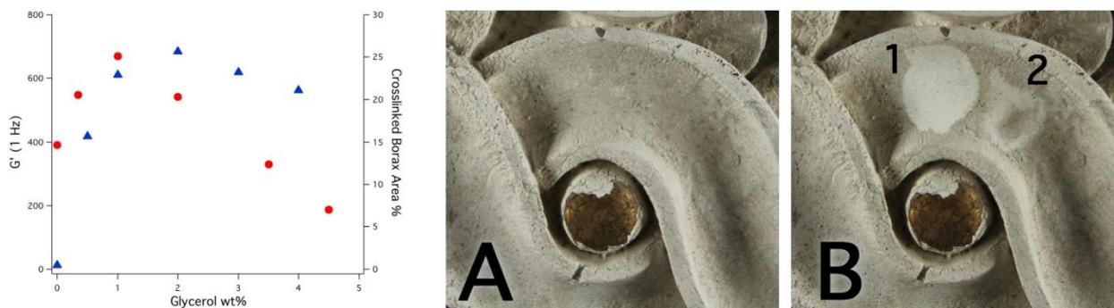
Figure 3: On the left, Storage modulus values at Frequency=1Hz (■) and Crosslinked Borate Area obtained from NMR measurements (▲) are plotted against glycerol concentration. Pictures on the right show the *stucco* surface before (A) and after (B) the cleaning, with the comparison between the the HPG based system (1) and a wet cotton swab (2).
